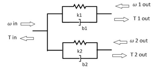
$$\begin{split} T_{in} &= -(\omega_{in} - \omega_{1out})b_1 - (\omega_{in} - \omega_{2out})b_2 - \theta_1 k_1 - \theta_2 k_2 \\ T_{1out} &= (\omega_{in} - \omega_{1out})b_1 + \theta_1 k_1 \\ T_{2out} &= (\omega_{in} - \omega_{2out})b_2 + \theta_2 k_2 \\ \dot{\theta}_1 &= (\omega_{in} - \omega_{1out}) \\ \dot{\theta}_2 &= (\omega_{in} - \omega_{2out}) \end{split}$$
