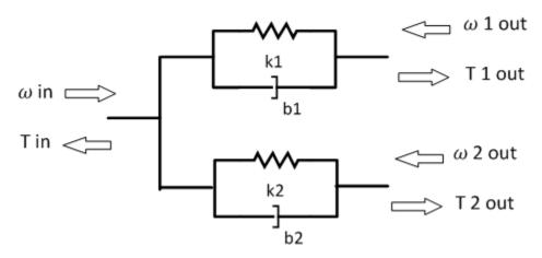
$$\begin{split} T_{out} &= (-\omega_{out} + \omega_{1in})b_1 + (-\omega_{out} + \omega_{2in})b_2 + \theta_1k_1 + \theta_2k_2 \\ T_{1out} &= (\omega_{out} - \omega_{1in})b_1 - \theta_1k_1 \\ T_{2out} &= (\omega_{out} - \omega_{2in})b_2 - \theta_2k_2 \\ \dot{\theta}_1 &= (\omega_{1in} - \omega_{out}) \\ \dot{\theta}_2 &= (\omega_{2in} - \omega_{out}) \end{split}$$
