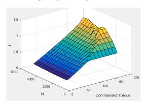
• The intake cam phaser angle command lookup table,  $f_{ICPCMD}$ , is a function of the engine load and engine speed
