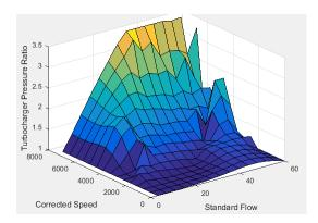
To calculate the standard air mass flow through the turbocharger, the block uses conservation of mass, the estimated intake port, and EGR mass flows (from the last estimated calculation). The calculation assumes negligible exhaust manifold filling dynamics.
