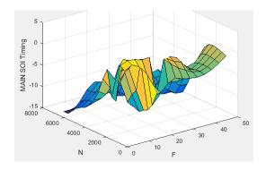
Fuel main injection timing fuel breakpoints, f\_main\_soi\_f\_bpt — Breakpoints
