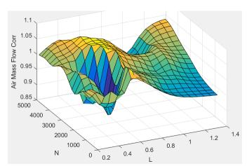
$\dot{m}_{intkideal}$  is engine intake port mass flow at arbitrary cam phaser angles, in g/s.
