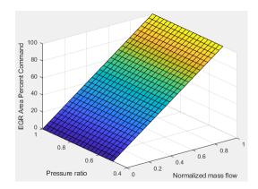
Open EGR valve standard flow, f\_egr\_max\_stdflow — Breakpoints
