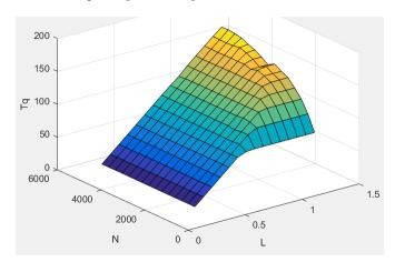
The simple torque lookup model assumes that the calibration has negative torque values to indicate the non-firing engine load (L) versus speed (N) condition. The calibrated table (L-by-N) contains the non-firing data in the first table row (1-by-N). When the fuel delivered to the engine is zero, the model uses the data in the first table row (1-by-N) at or above 100 AFR. 100 AFR results from fuel cutoff or very lean operation where combustion cannot occur.
